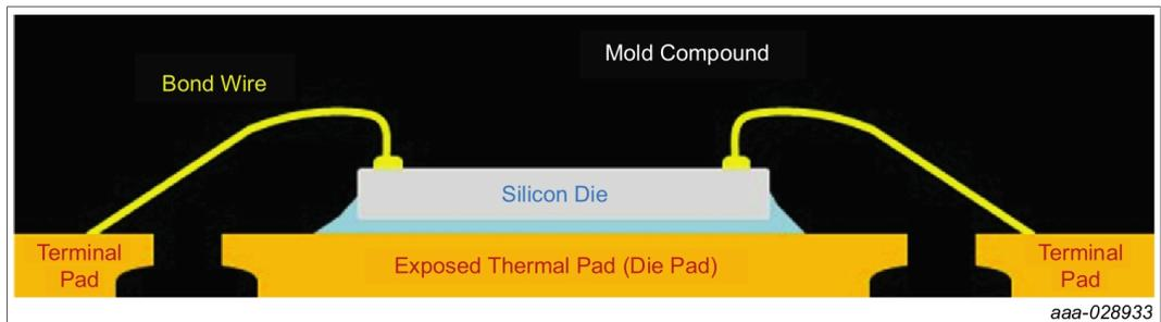
Figure 4. Cross-section of a sawn QFN with exposed pad
